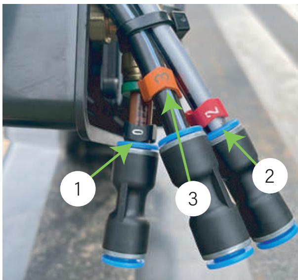
1. Supply Pressure - "0" 2. Row Cleaner Raise - "2" 3. Row Cleaner Lower - "3"
